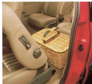
With a forward-folding driver's seatback, access to the second row is an easy proposition.
